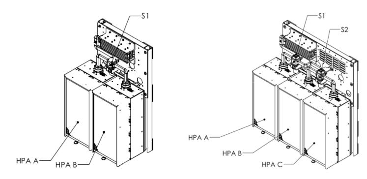
Installation of ETL redundant systems and power amplifiers is easy. The light-weight, modular design enables installation by a single person, even in some of the most difficult to access applications. Simply remove the amplifier from its shipping container, install a single mounting bracket and slide into the system. Secure the waveguide quick connect then lock the bracket and plug in the cables. The amplifier is ready for a quick software configuration for the system and ready for use.
