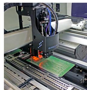
ETL's twin head pick and place machine, capable of placing 32,000 components per hour
