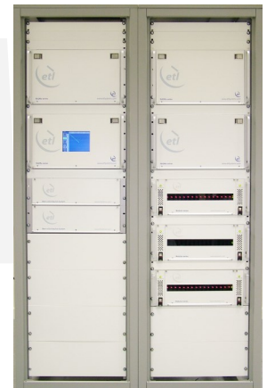
64 x 64 Enigma system with splitters & combiners
