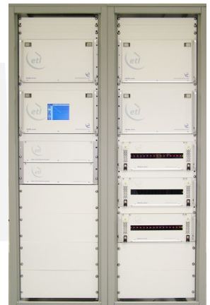
64 x 64 Enigma system with splitters & combiners
