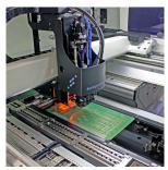
ETL's twin head pick and place machine, capable of placing 32,000 components per hour
