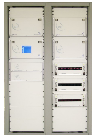
64 x 64 Enigma system with splitters & combiners
