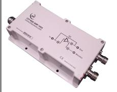
CST-BAE-AMP-1033 is a custom designed L-band ODU amplifier with 25 dB gain over 950 to 2000 MHz and Bidirectional DC and 10 MHz pass on the through path. It also has an integrated -25dB Coupled port with DC block.
