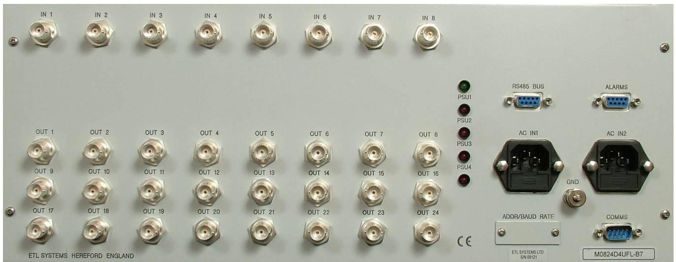
Rear View of Model M0824D4UFL with 75 ohm BNC connectors
