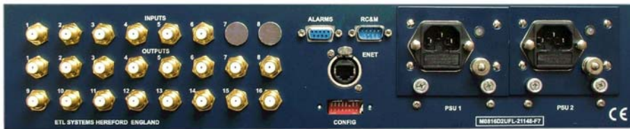
Fig 2 – Showing similar matrix rear panel, part populated as 6 x 16. Note hot swap PSU modules; and serial and Ethernet remote control ports.
