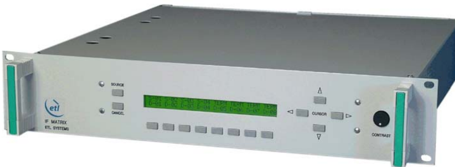
Picture of Front & Rear Panel of 8x8 IF Matrix
