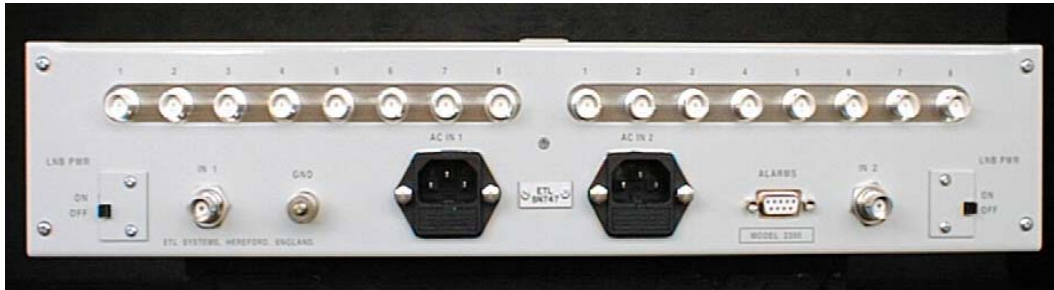
Photo of similar 2U dual 8-way splitter with BNC connectors and LNB powering
