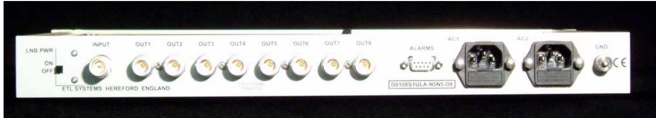
Photo of rear panel of similar 8 way splitter
