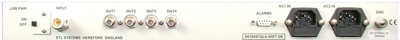
Rear view of similar model with 50 ohm N-type connectors (IN) and 75 ohm F-type connectors (OUT)
