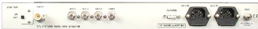
Rear view of a similar 4-way L-band Active Splitter showing switchable LNB Powering
