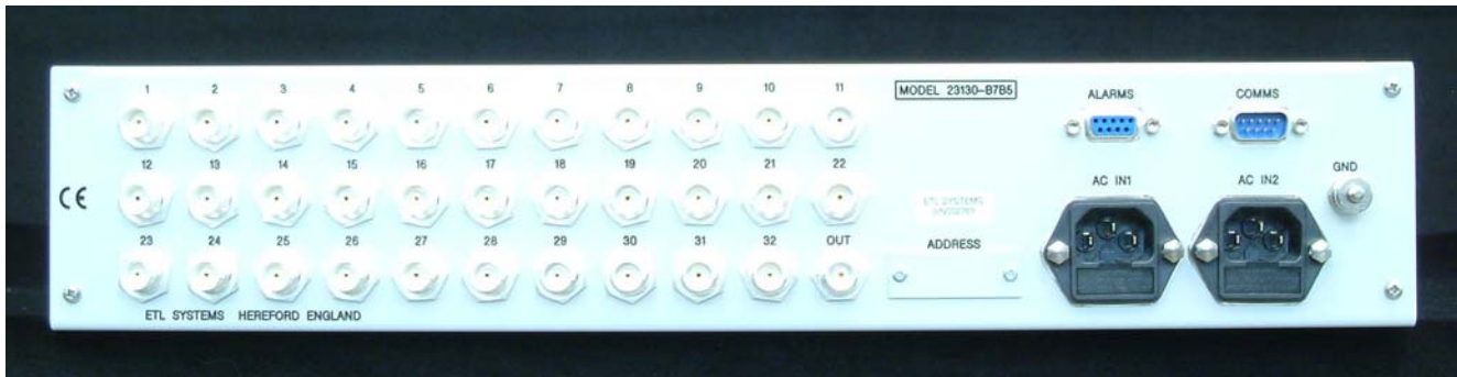
Fig. 2 – 2U model 23130 32x1 switch – rear view showing serial port for remote control.
