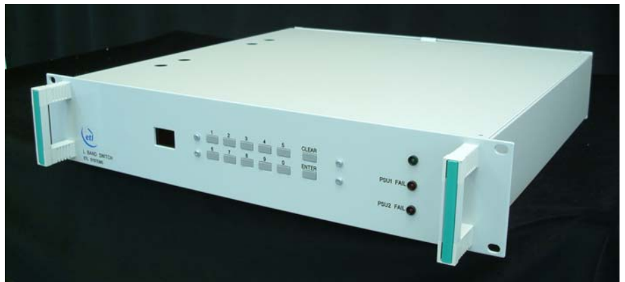
Fig. 1 – 2U model 23130 32x1 switch shelf with integrated controller and RS232 / 485 remote control.
