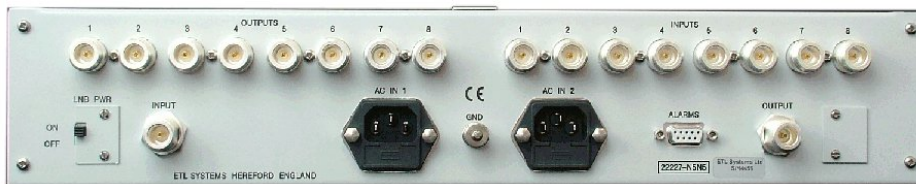
Front & Rear View of an 8-way Combiner & Splitter with LNB Powering
