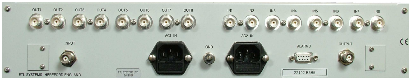
Rear View of Model 22192 with 50 ohm BNC connectors
