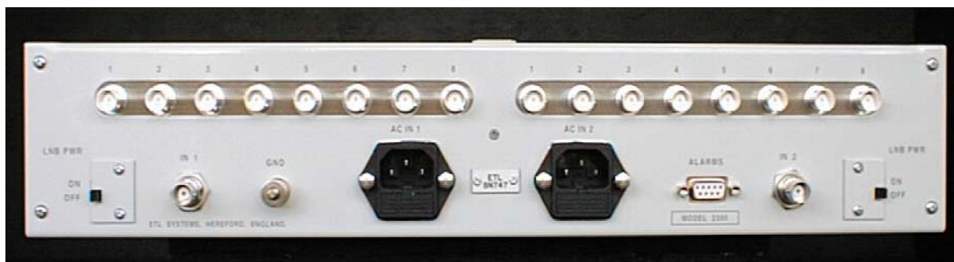
Photo of similar 2U dual 8-way splitter with BNC connectors
