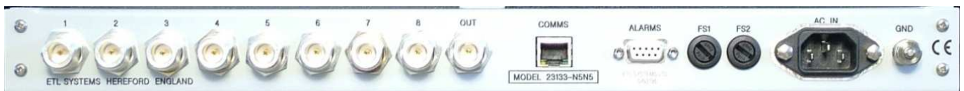
Rear View of Model 23133 with 50 ohm N-type connectors
