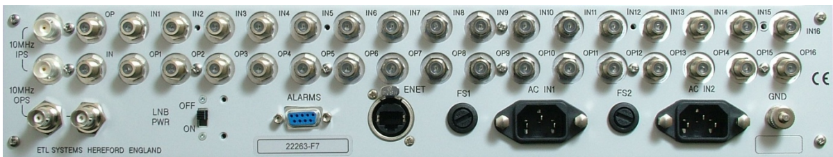
Rear View of a 16-way Hybrid Splitter/Combiner showing switchable LNB powering, 10MHz Ports, dry contact alarm port and Ethernet monitoring port
