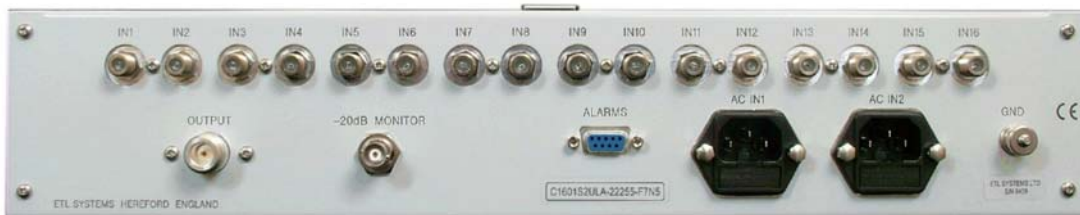
Rear View of a 16-way L-band Combiner showing the -20dB Monitor Port
