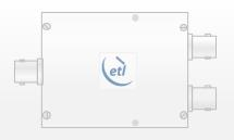
10dB L-band proximity coupler with DC and 10MHz pass between input and transmit ports. The coupled port is DC blocked.
